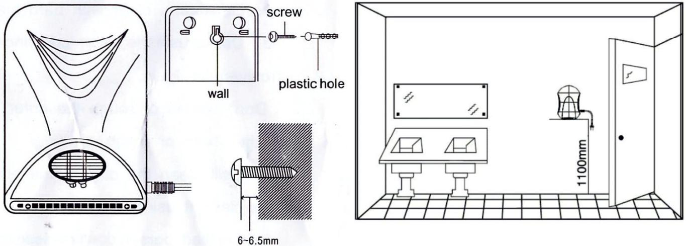
1. The appliance must be installed at a height of about 1.1 meters from the floor and far from other objects. In particular, the towels should be at least one meter away from sink or from possible splashing. Even below unit there must be no objects, because they could dell'asciugamani be ruined by heat.
